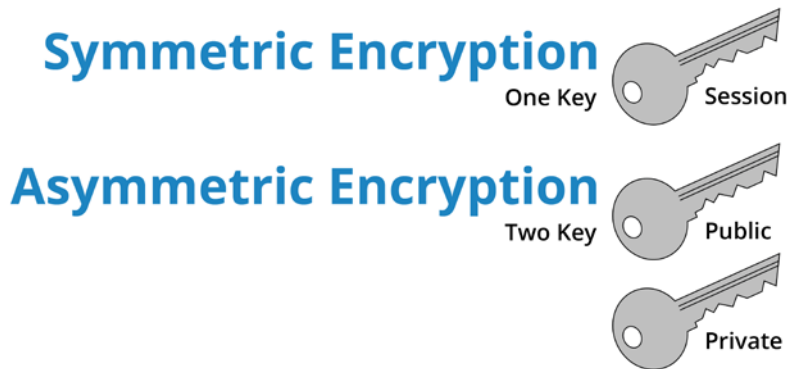
Figure 1.4: Symmetric encryption uses one key while asymmetric encryption uses two keys
