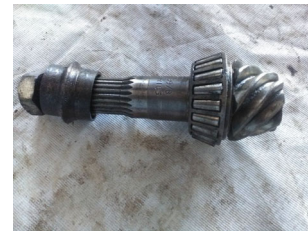
Figure 3 Test spiral bevel crown pinion from differential gear box
