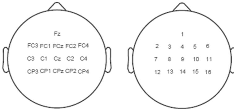
**Fig. 6** Layout of the used 16 EEG channels cap
