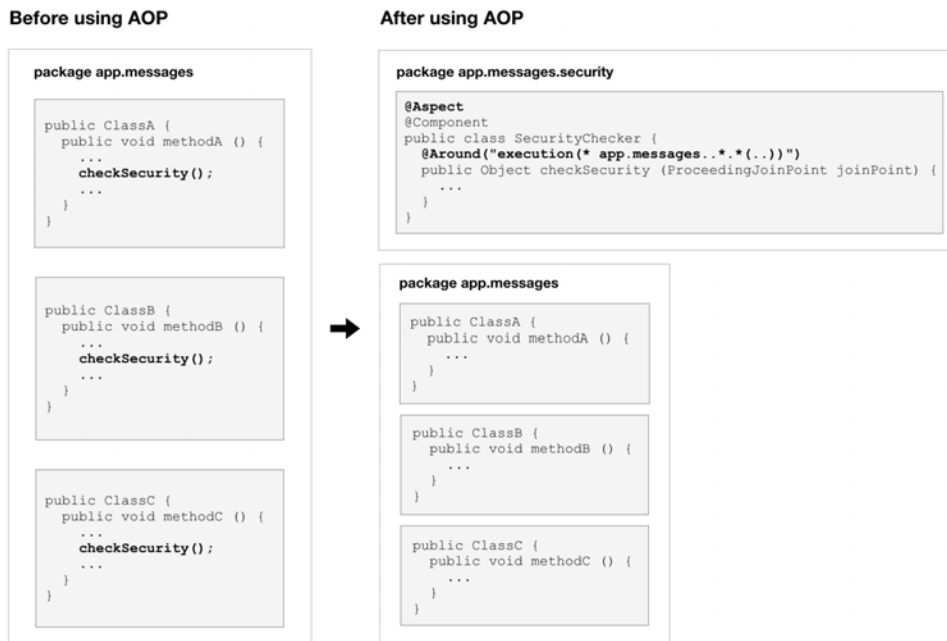
Figure 3.7: AOP for security checking
