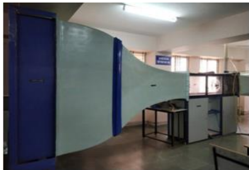
Figure 3. Wind tunnel test rig with scaled bus model
