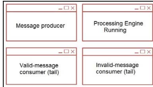
Figure 3.3: The four terminal windows to test the processing engine including: message producer, valid message consumer, invalid message consumer, and the processing engine itself
