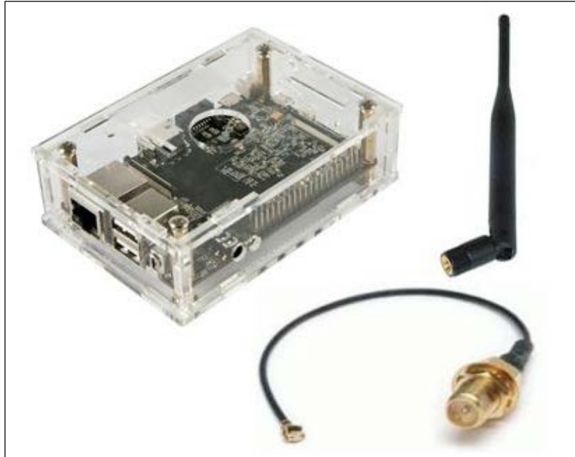
Figure 31: The Banana Pro acrylic case with the 5 dBi antenna and R-SMA connector (source: the Allnet shop)
