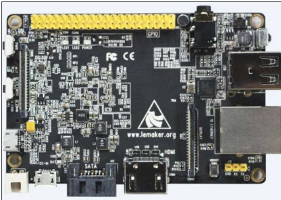
Figure 1: Banana Pro is a dual core computer featuring many connectors (source: http://en.wikipedia.org/wiki/Banana_Pro ).
