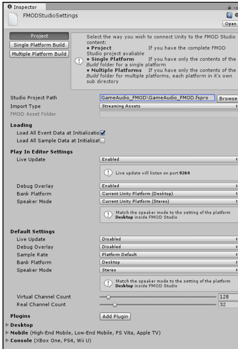
Inspector window showing properly configured FMOD Studio Project settings
