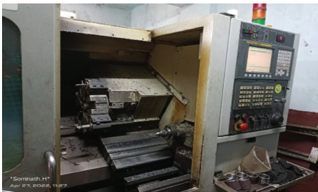
a. CNC lathe used for turning operation.
