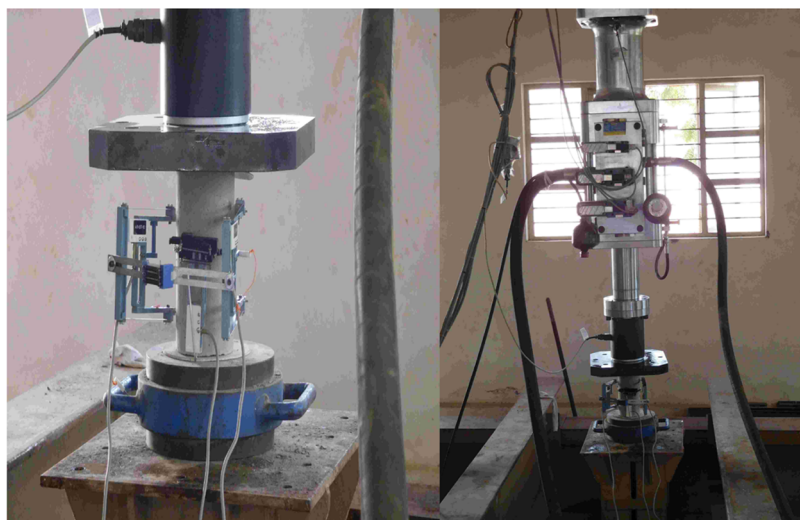
Figure 4. Apparatus to test cylinder specimens.
