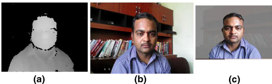
Fig. 9 Background segmented world image (a) Depth image (b) Color Image (c) Background separated image
