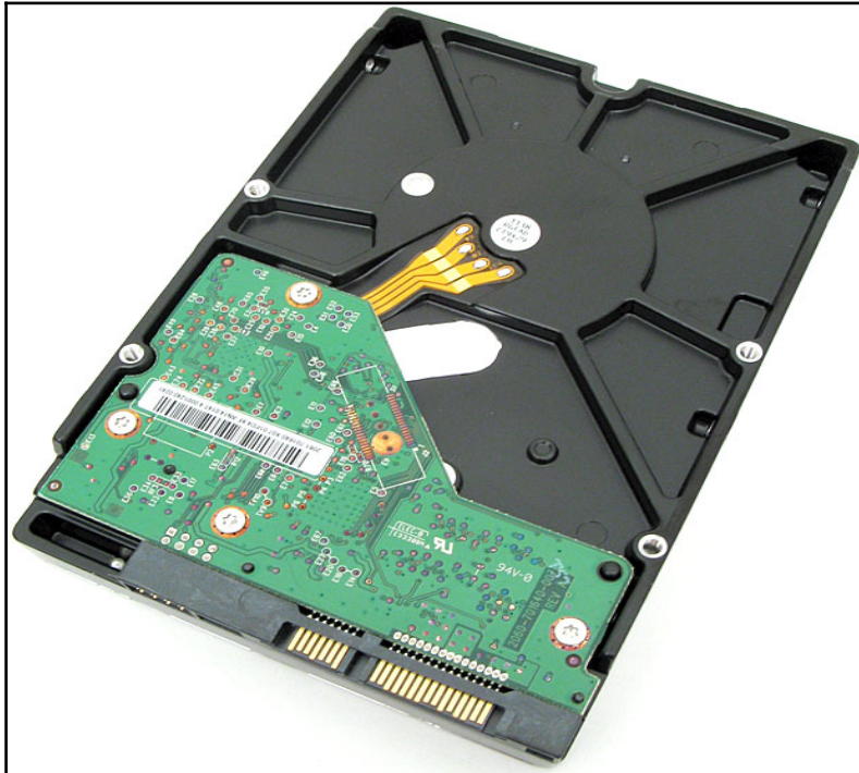
Visualizing a hard disk with a SATA interface and disk buffer on the control board
