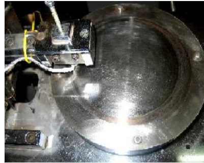
Figure 3.5 Friction temperature wear measurement and wear track on disc
