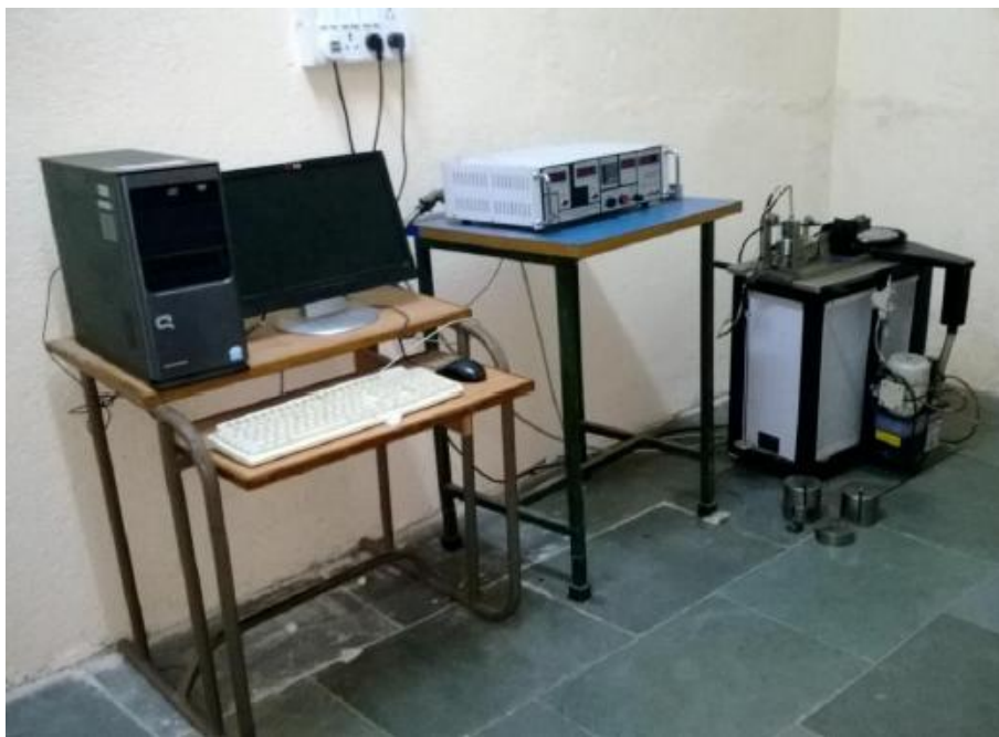
Figure 3.6 DUCOM pin-on-disc wear testing machine (TR-20-LE)
