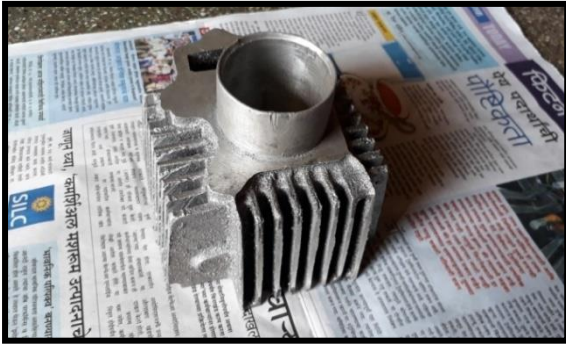
Figure 5.41, Photography of semi-finished casting, right side machined
