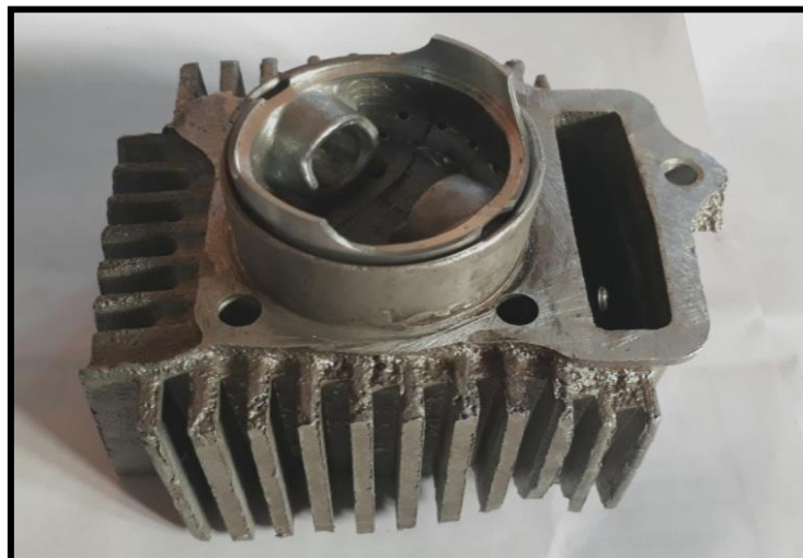
Figure 5.51, Photography of finished casting with piston in bore, bottom view
