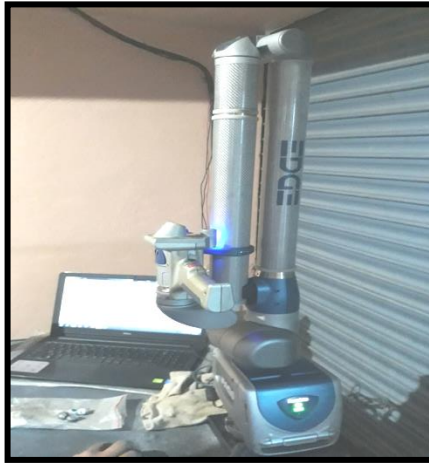
Figure 5.52, Photographic view of Faro Make 3D Scanner
