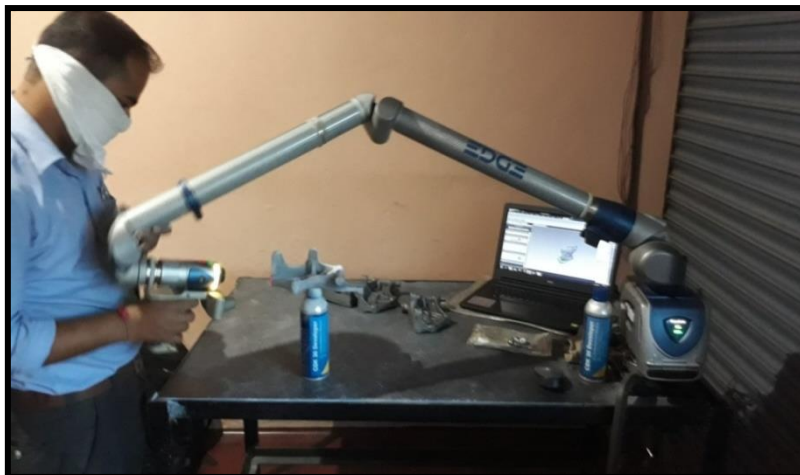
Figure 5.54, Photographic view during scanning of component
