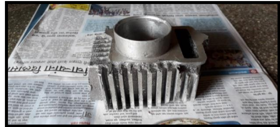
Figure 5.38, Photography of semi-finished casting, fins machined
