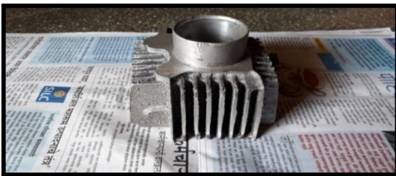
Figure 5.37, Photography of semi-finished casting, lower surface machined
