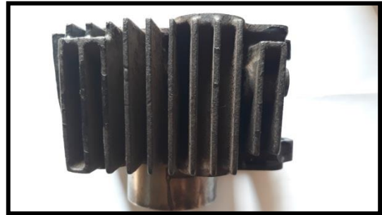
Figure 5.20, C. I. block, Side View
