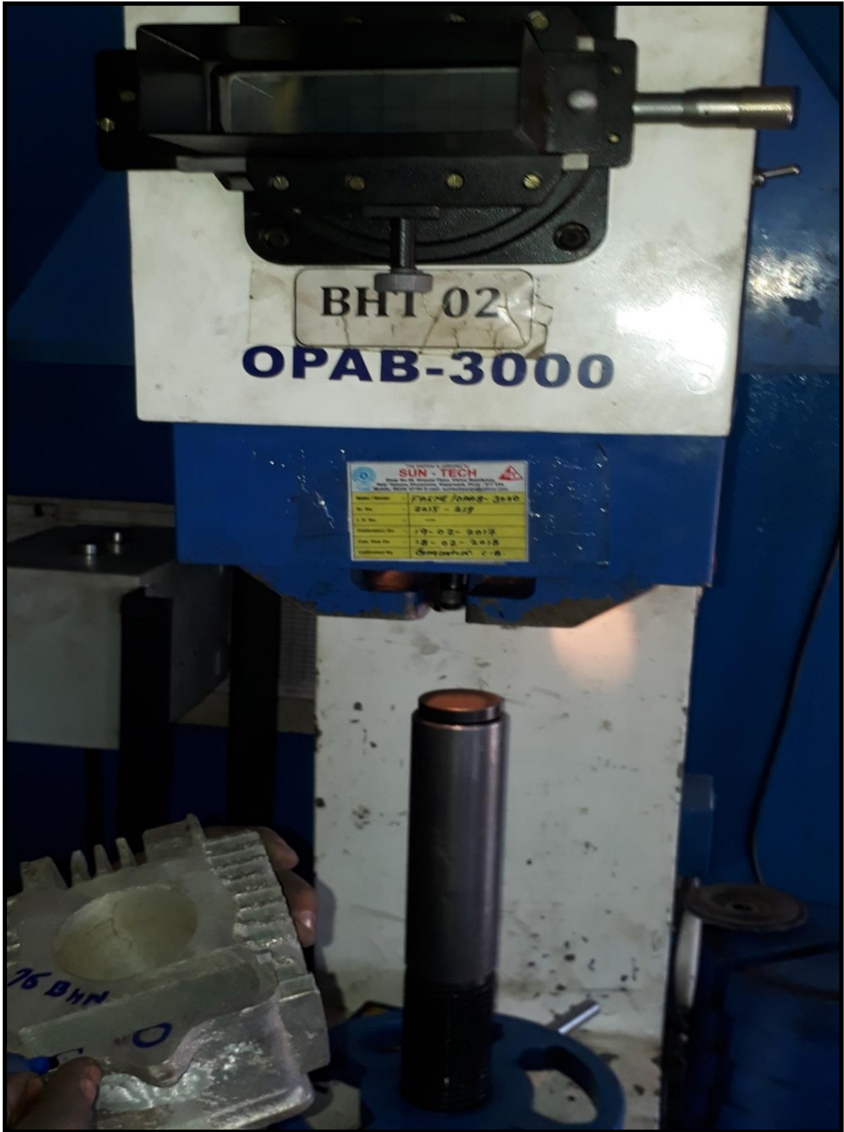
Figure 5.47, Photography of casting post heat treatment showing hardness
