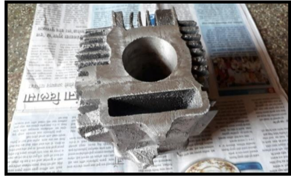
Figure 5.42, Photography of semi-finished casting, top face machined
