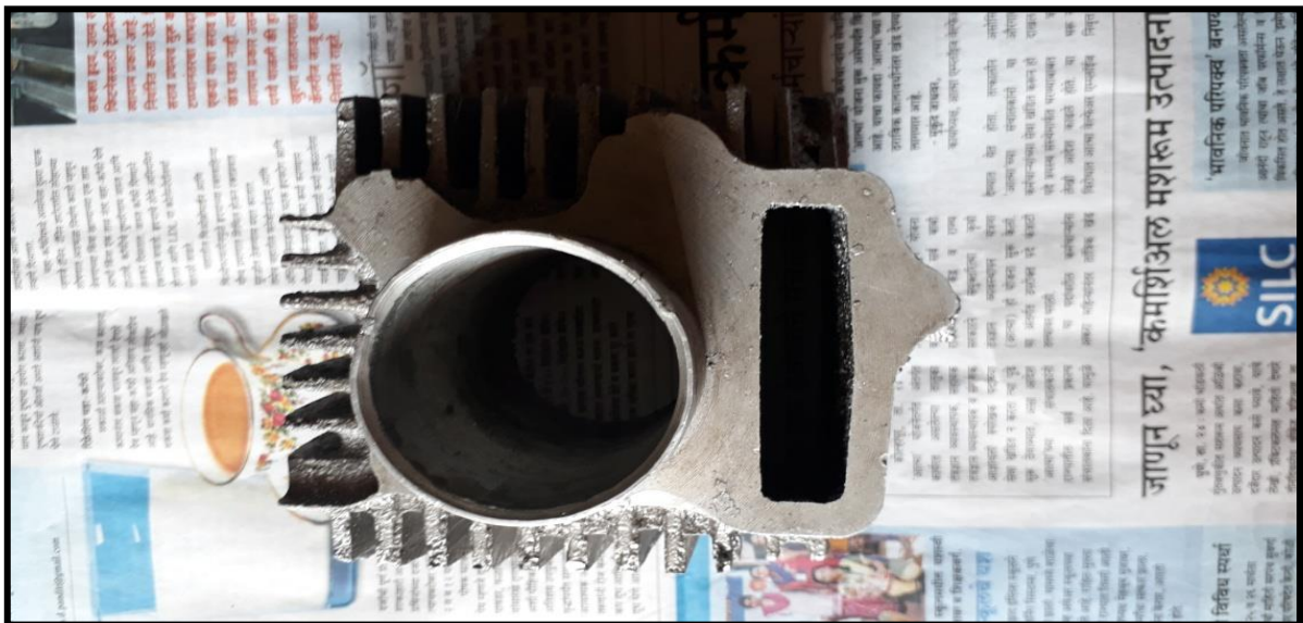
Figure 5.43, Photography of semi-finished casting, top face machined
