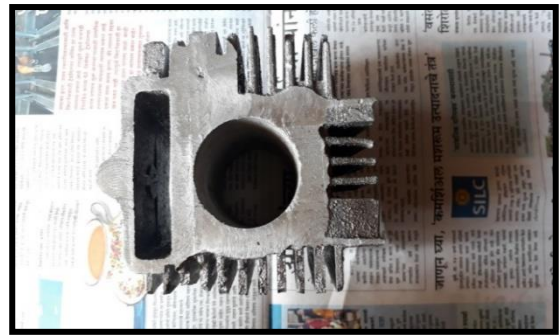
Figure 5.44, Photography of semi-finished casting, top face machined
