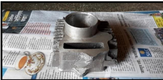
Figure 5.39, Photography of semi finished casting, Left side machined
