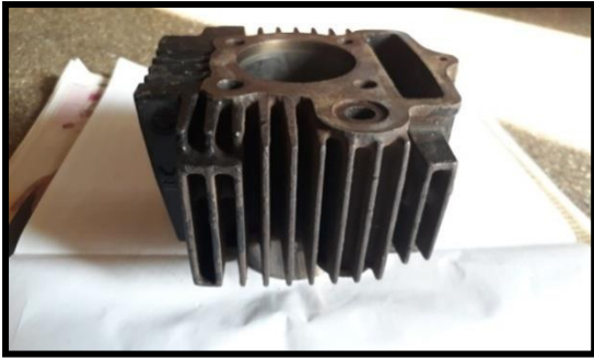
Figure 5.25, C. I. block, top and side wall
