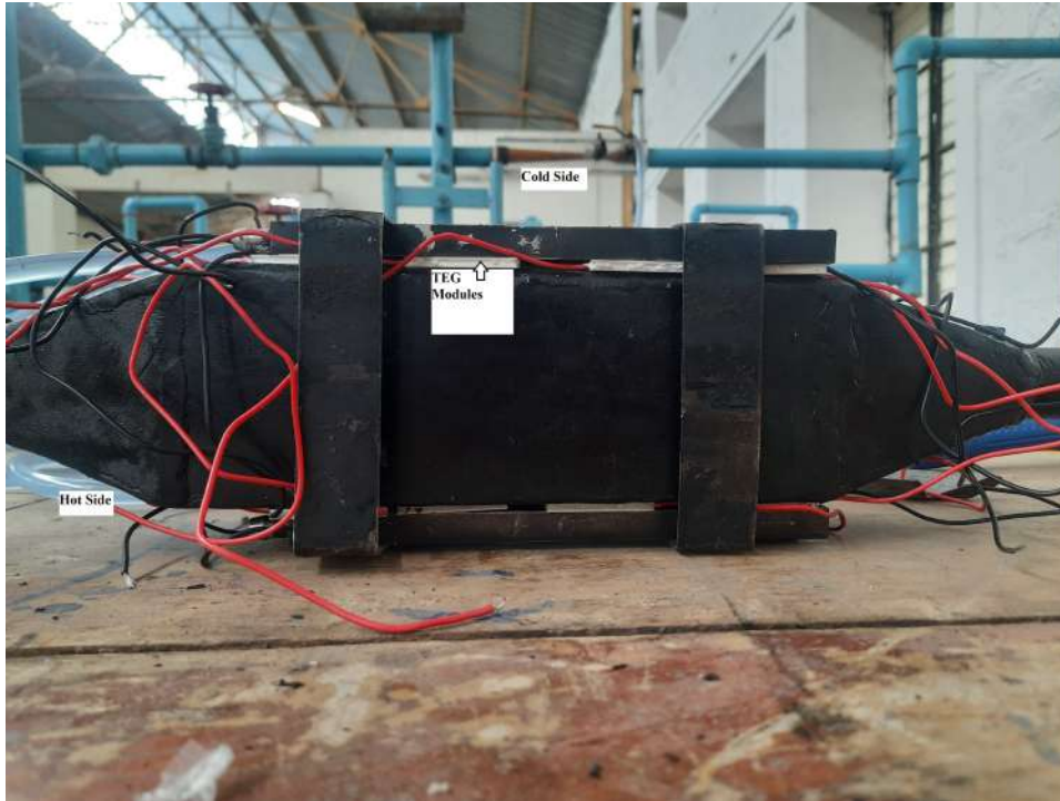
Figure 4.42: Heat Exchanger for hot air blower
