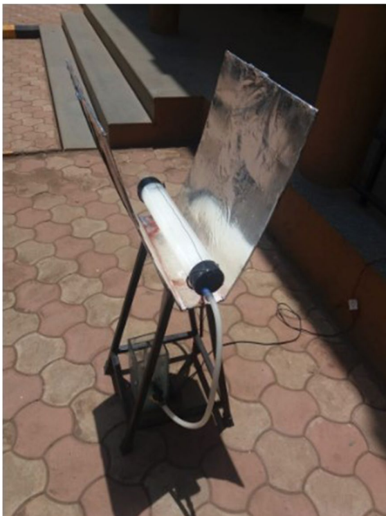
Fig. 2 CPC of reflective surface covered with aluminum foil
