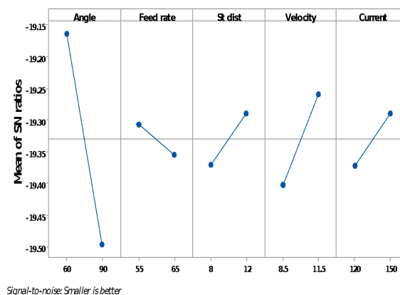
Figure 5: Main Effect Plot of S/N Ratio Based on Data Means of Back Height
