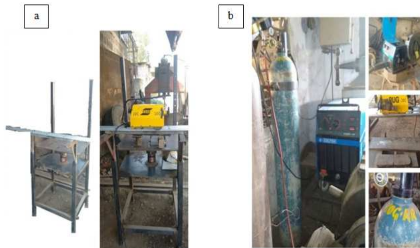
Figure 3: (a) Arrangement of Setup Table Along with Pug Cutting Machine (b) Welding Machine and Shielding Gas Tank Along with Welding Wire Spool
