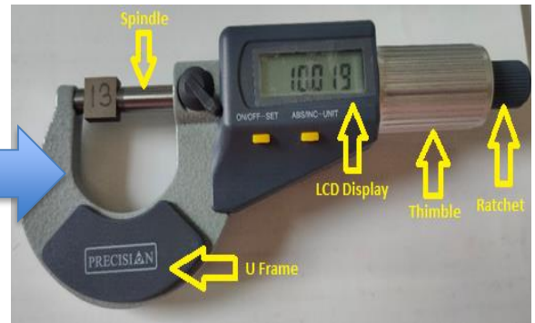
10. Measurement of dimensional deviation using digital micrometer
