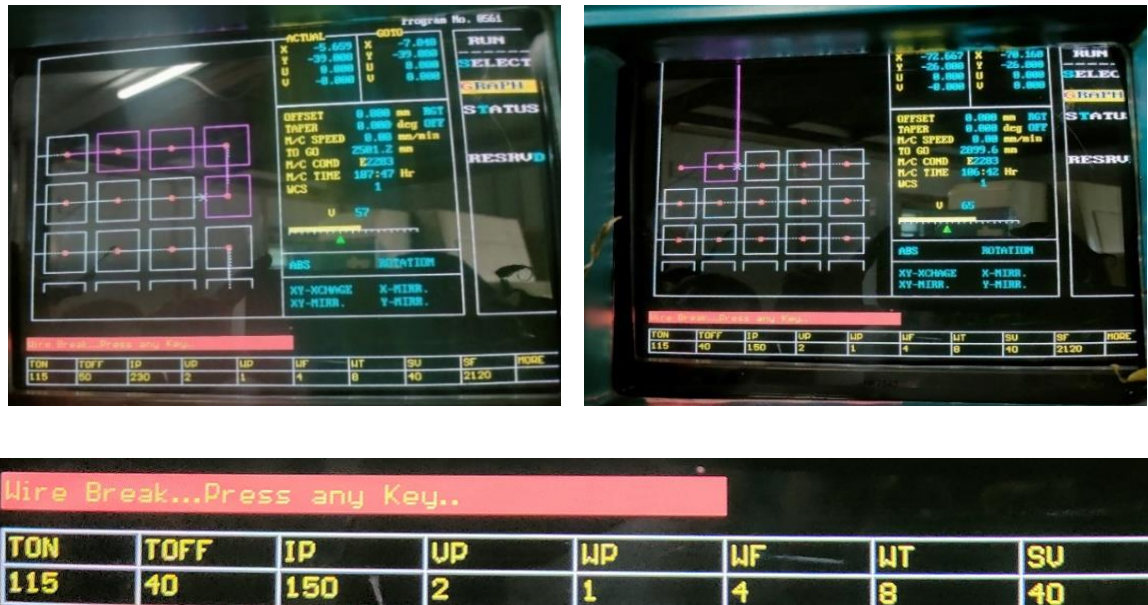
Figure 4.4 Machine display showing wire breakage warning
