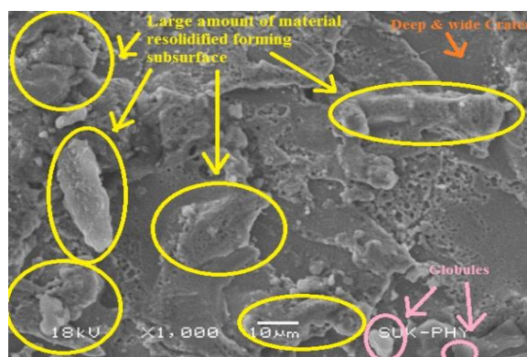
Figure 4.15 SEM image for machined surface using Gamma Coated wire
