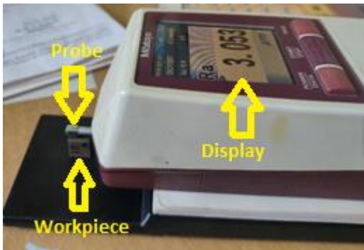
9. Measurement of surface roughness using surface roughness tester
