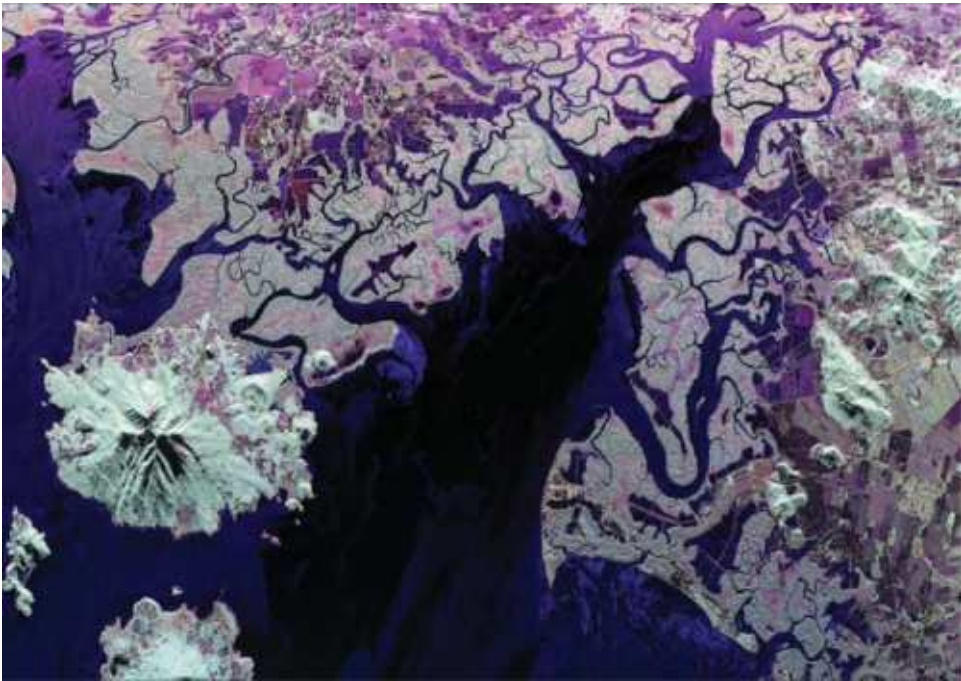
Plate 24 Polarimetric L-band radar images acquired from an uninhabited aerial vehicle (UAV). (a) Hofjokull (glacier), Iceland, June. Nominal scale 1:125,000. (b) Bahia de San Loranzo, Honduras, February. Nominal scale 1:300,000. (Courtesy NASA/JPL/Caltech.) (For major discussion, see Section 6.8.)
