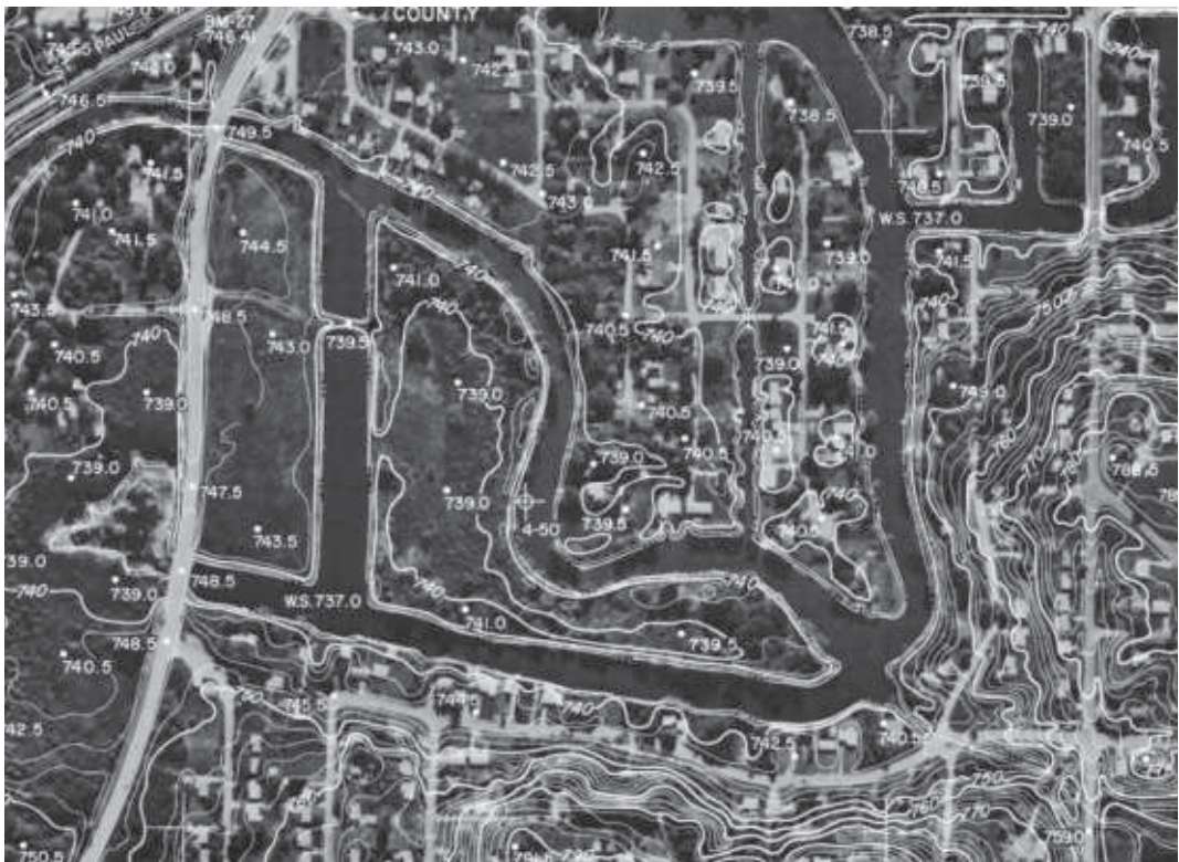
Figure 3.28 Portion of a 1:4800 topographic orthophotomap. Photography taken over the Fox Chain of Lakes, IL. (Courtesy Alster and Associates, Inc.)
