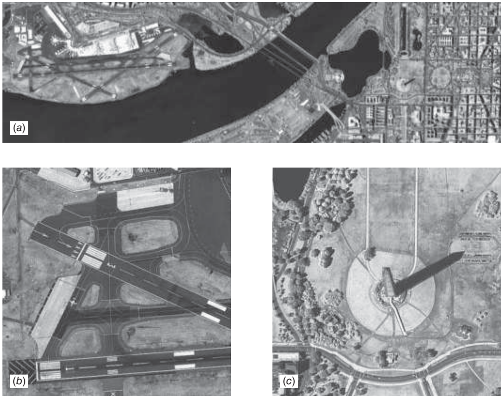
Figure 5.27 First IKONOS image, acquired on September 30, 1999, over Washington, DC: (a) Panchromatic image; (b) enlargement showing runway at Ronald Reagan Washington National Airport; (c) enlargement showing Washington Monument (with scaffolding present during renovation activity). (Courtesy DigitalGlobe.)
