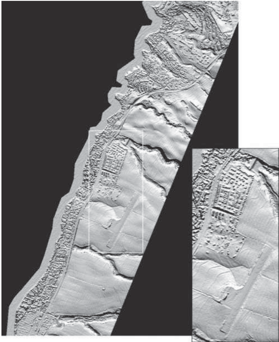
Figure 6.63 Shaded-relief DEM from Leica Geosystems ALS-40 Airborne Laser Scanner data, West Maui, Hawaii. Scale 1:48,000 (main image), 1:24,000 (inset). (Courtesy NOAA Coastal Services Center.)
