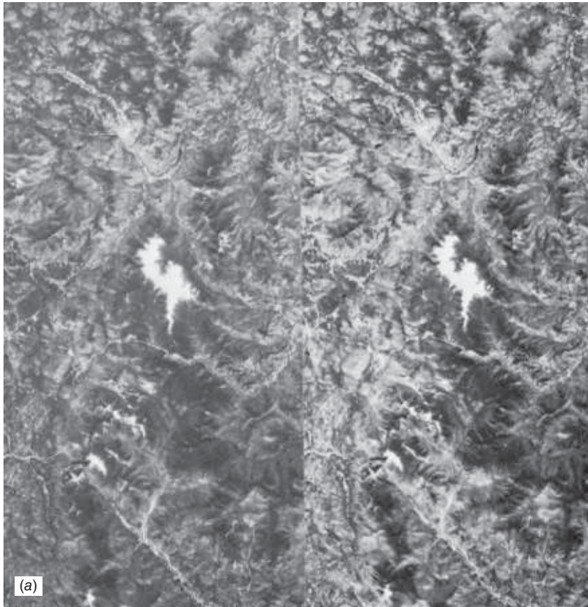
Figure 3.4 Large Format Camera stereopairs, Mt. Washington and vicinity, New Hampshire; scale 1:800,000 (1.5 times enlargement from original image scale): (a) 0.30 base–height ratio; (b) 1.2 base–height ratio. (Courtesy NASA and ITEK Optical Systems.)
