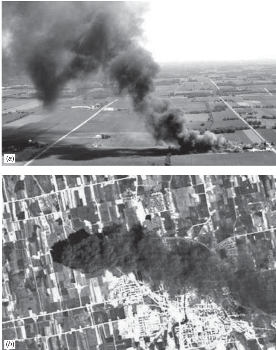
Figure 8.29 Massive smoke plume rising from a fire at a tire recycling facility in Watertown, WI. (a) Oblique airphoto looking to the south. (Courtesy Mike DeVries/The Capital Times.) (b) Landsat Thematic Mapper image (north is to the top). Scale 1:97,000. (a) and (b) are images from the same day, but are not simultaneous. (Author-prepared figure.)
