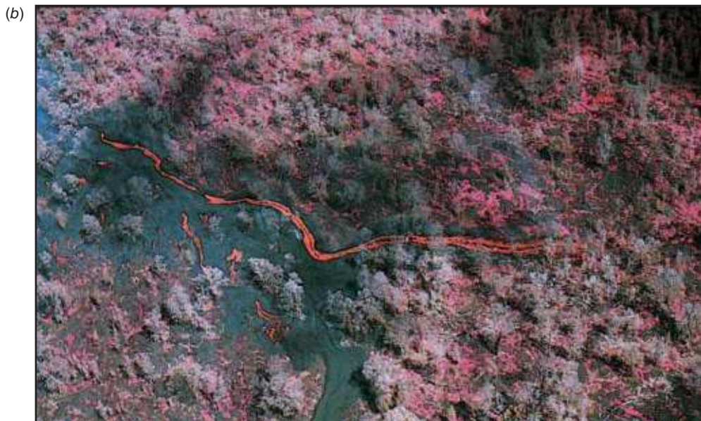
Plate 5 Oblique normal color (a) and color infrared (b) aerial photographs showing flowing lava on the flank of Kilauea Volcano, Hawaii. The orange tones on the color infrared photograph represent infrared energy emitted from the flowing lava. The pink tones represent sunlight reflected from the living vegetation. (Author-prepared figure.) (For major discussion, see Section 2.4.)
