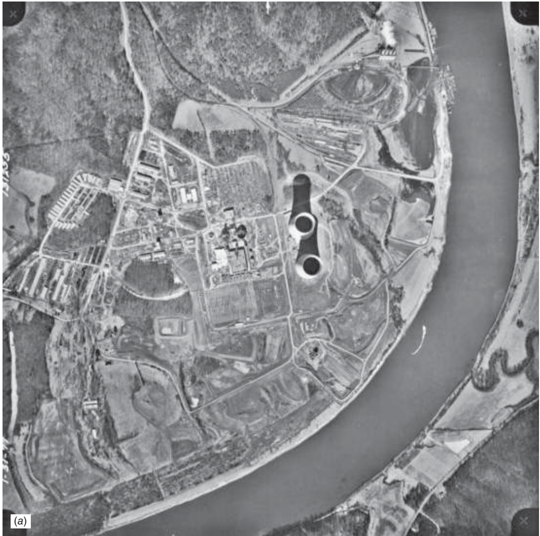
Figure 3.11 Vertical photographs of the Watts Bar Nuclear Power Plant Site, near Kingston, TN. In (a) the two plant cooling towers appear near the principal point and exhibit only slight relief displacement. The towers manifest severe relief displacement in (b). (Courtesy Mapping Services Branch, Tennessee Valley Authority.)
