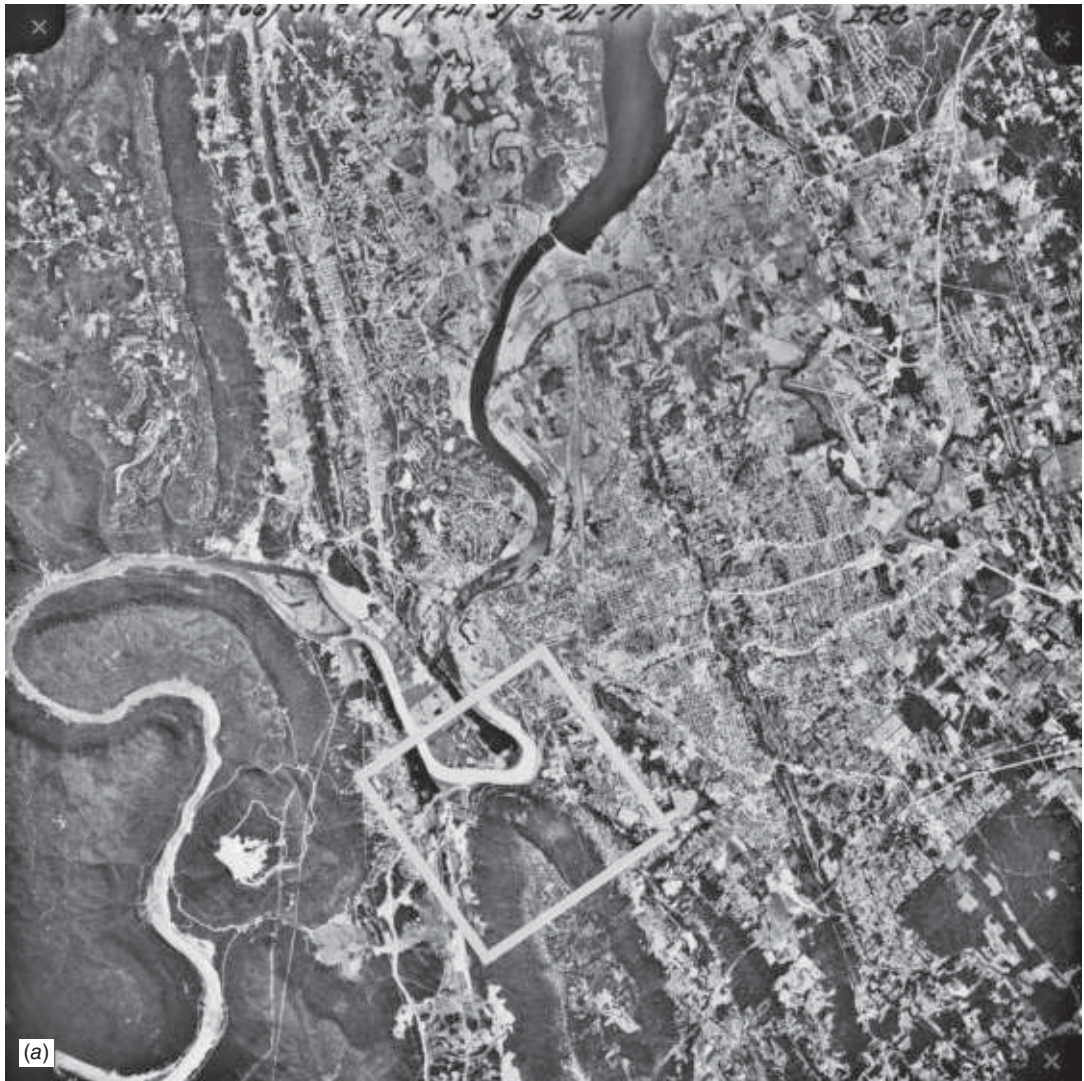
Figure 3.9 (a) Scale 1:210,000 vertical aerial photograph showing Chattanooga, TN. This figure is a 1.75 \times reduction of an original photograph taken with f = 152.4 mm from 18,300 m flying height. (NASA photograph.) (b) Scale 1:35,000 vertical aerial photograph providing coverage of area outlined in (a). This figure is a 1.75 \times reduction of an original photograph taken with f = 152.4 mm from 3050 m flying height. (c) Scale 1:10,500 vertical aerial photograph providing coverage of area outlined in (b). This figure is a 1.75 \times reduction of an original photograph taken with f = 152.4 mm from 915 m flying height. (Courtesy Mapping Services Branch, Tennessee Valley Authority.)
