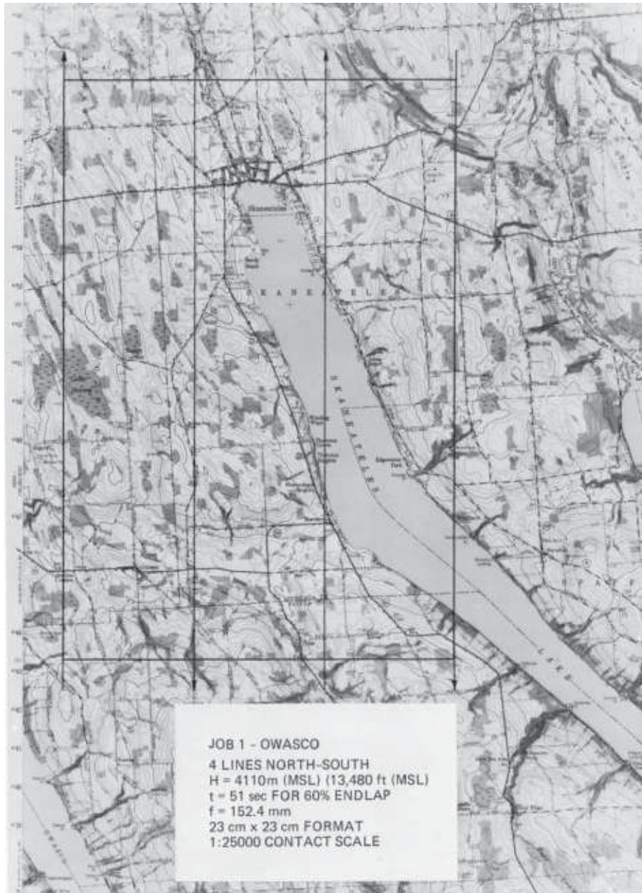
Figure 3.34 Flight map for Example 3.11. (Lines indicate centers of each flight line to be followed.) (Author-prepared figure.)
