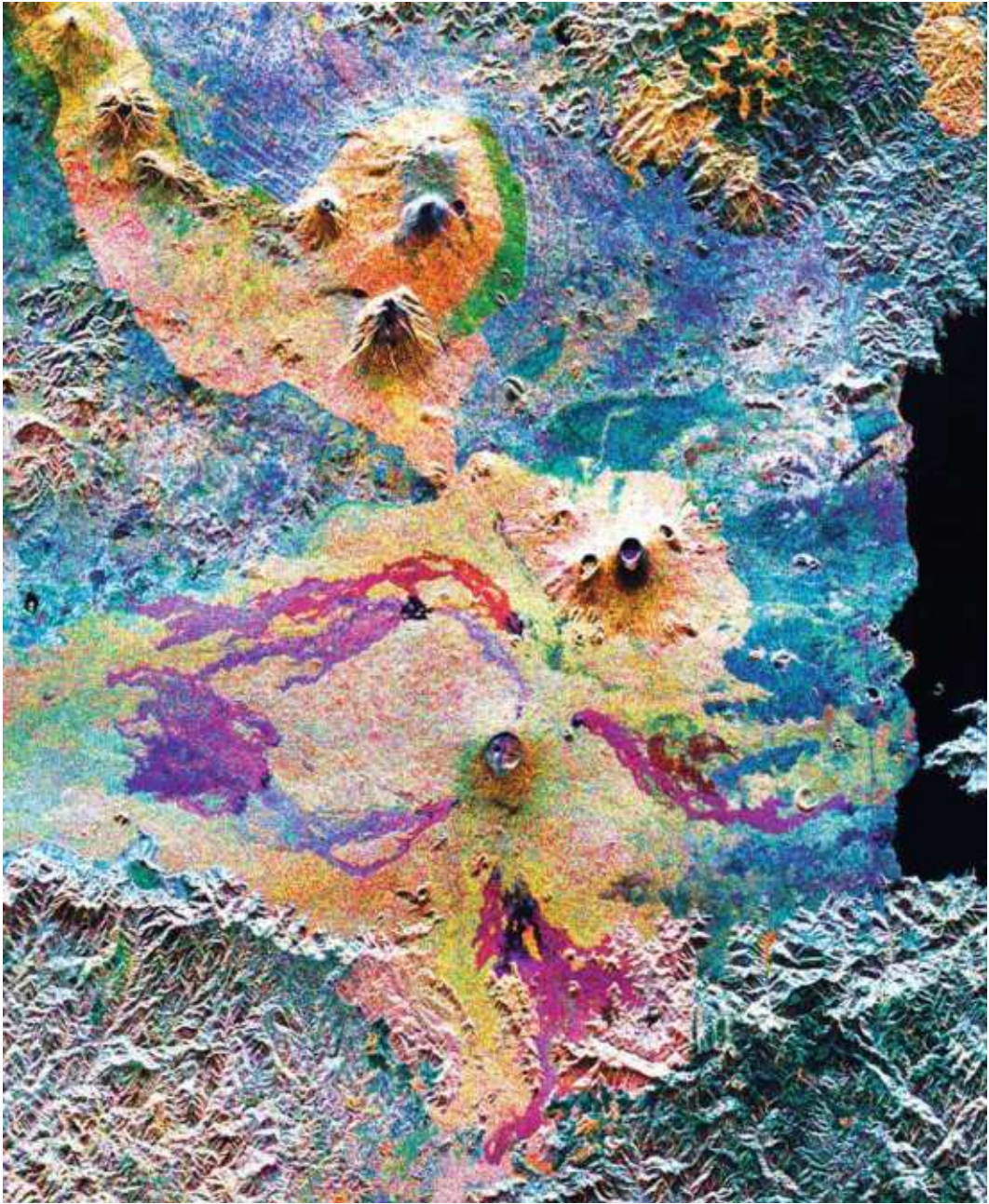
Plate 26 SIR-C color composite SAR image of a volcano-dominated landscape in central Africa, October 1994. Scale 1:360,000. (Courtesy NASA/JPL/Caltech.) (For major discussion, see Section 6.11.)
