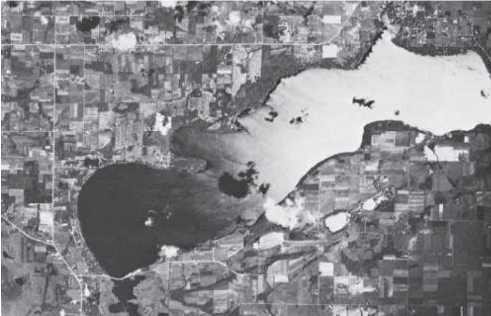
Figure 1.16 Aerial photograph containing areas of specular reflection from water bodies. This image is a portion of a summertime photograph taken over Green Lake, Green Lake County, WI. Scale 1:95,000. Cloud shadows indicate direction of sunlight at time of exposure. Reproduced from color IR original. (NASA image.)
