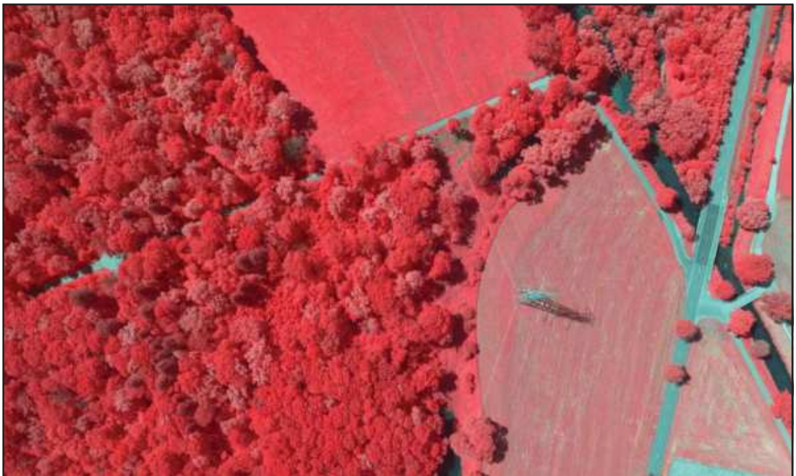
Plate 6 Color (a) and color infrared (b) aerial photographs taken with a Leica RCD30 medium-format digital camera system in support of a power line corridor mapping project. (Courtesy Leica Geosystems, Geospatial Solutions Division.) (For major discussion, see Section 2.6.)
