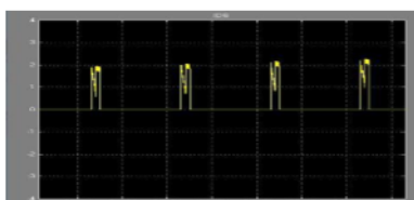
7.7 current flows in Diode D6
