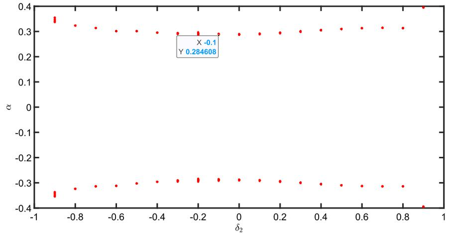
**Fig. 20** Comparative bifurcation diagram of the system response with tuned  $\delta_2$ , with insets of time histories of (a) Dynamics in aperiodic regime (b) Stall flutter amplitude reduction
