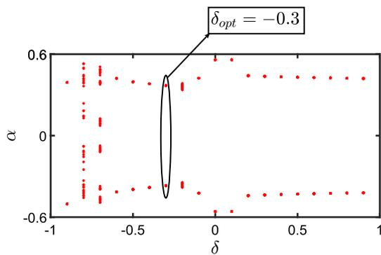
**Fig. 8** Peak pitch amplitude  $\alpha$  vs NES offset  $\delta$
