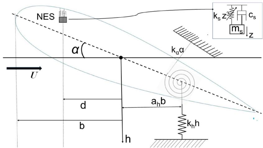
mid-chord, while the centre of mass is located at a distance  $\chi_\alpha b$  along the chord from the elastic axis.
