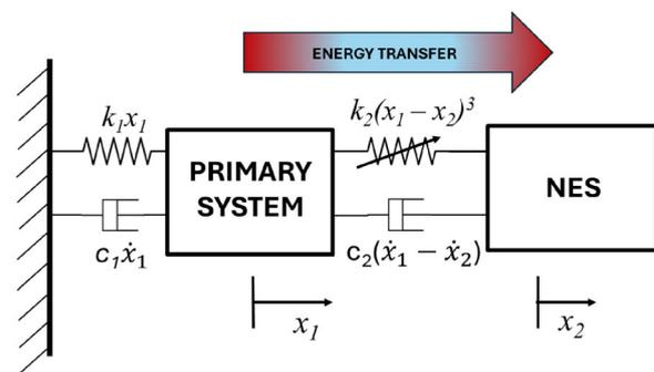
**Fig. 2** A sketch of a linear oscillator with NES attached.  $x_1$ ,  $\dot{x}_1$ ,  $x_2$  and  $\dot{x}_2$  are the state variables of the linear oscillator and NES respectively
