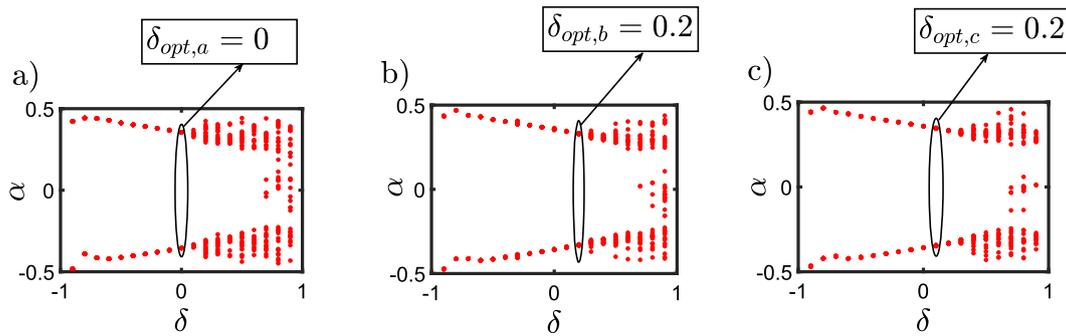
Fig. 11 Sweep results varying higher values of NES stiffness. Tuned  $\delta$  values for Cases **a**, **b** and **c** in Table 5 are also identified
