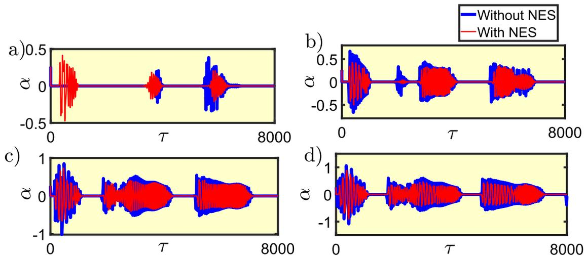
**Fig. 16** Response of system coupled with NES at (a)  $V_m = 5.6$ , (b)  $V_m = 6$ , (c)  $V_m = 6.6$ , (d)  $V_m = 7$  for a noise intensity of  $\sigma = 0.3$  and long time scale fluctuations
