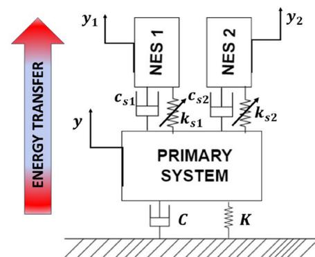
**Fig. 3** A representation of a primary system with two NESs attached in parallel. The energy transfer takes place from the region of higher concentration (primary system) to that of lower energy concentration (NESs)
