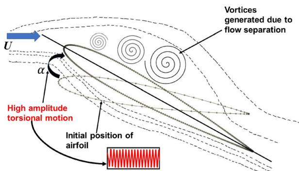
**Fig. 1** A schematic of stall instability and flow separation leading to high amplitude torsional oscillations in an airfoil. The streamlines represent the flow of air around the stalled airfoil. Stall instability consists of several stages or modules [8] eventually culminating in dangerous high amplitude stall flutter oscillations
