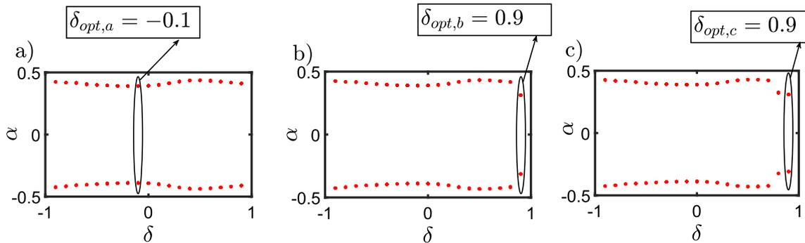
Fig. 12 Sweep Results using  $\lambda_s = 0.1$  and varying high values of NES stiffness. Tuned  $\delta$  values for cases **a**, **b** and **c** in Table 6 are also identified
