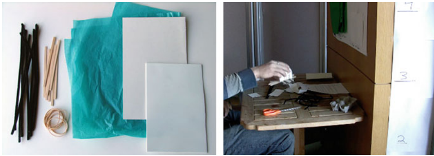
Fig. 1 Left: Materials constraints in the design task: pipe cleaners, popsicle sticks, rubber bands, tissue paper, poster board, and flat foam. Right: Experimental setup for the design exercise
