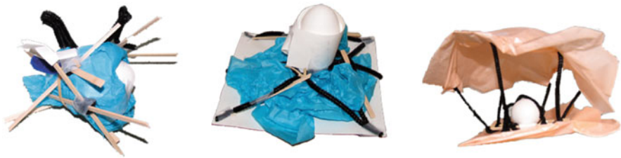
Fig. 9 Left: Participant 3 (iteration) successfully protected the egg at 5 ft. Middle: Participant 18 (iteration) protected at 2 ft. Right: Participant 28 (iteration) protected the egg only at 1 ft
