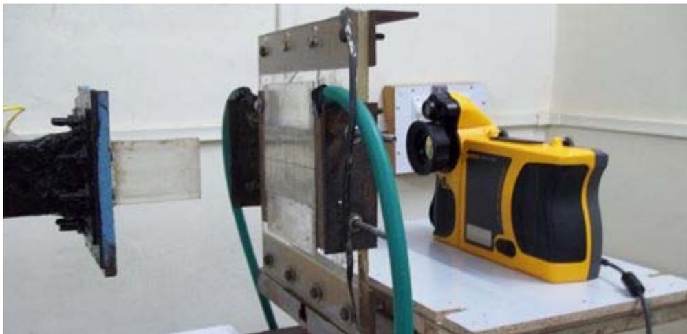
**Fig 5.16** Photograph of the set up showing the position of Slot Jet, Target Plate, and IR Camera.
