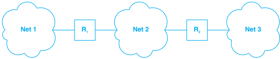
Figure 3.3 Three networks interconnected by two routers.
