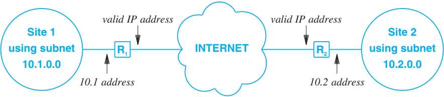
Figure 19.4 Example of a VPN that interconnects two sites over the global Internet while computers at each site use non-routable (i.e., private) addresses.
