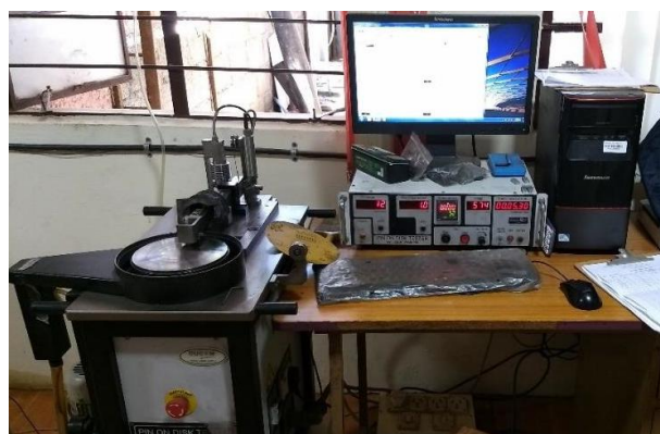
Fig. 5. Wear Testing apparatus for experimentation.
