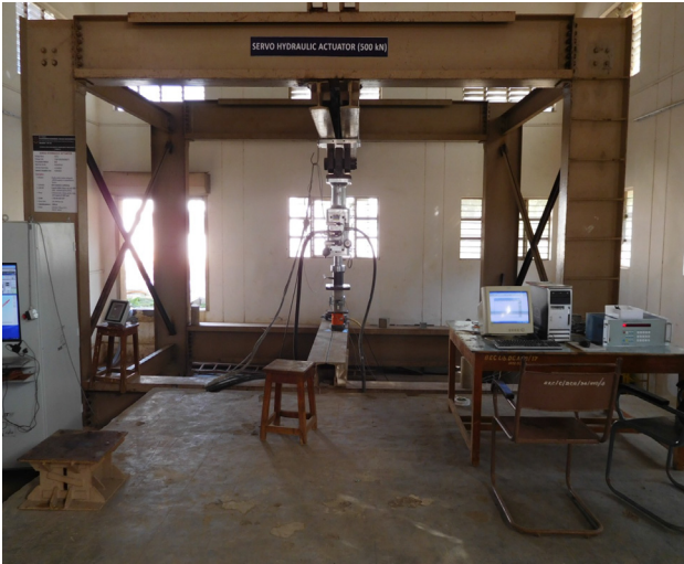
Fig. 1. Instrumentation to test GPC specimens.
