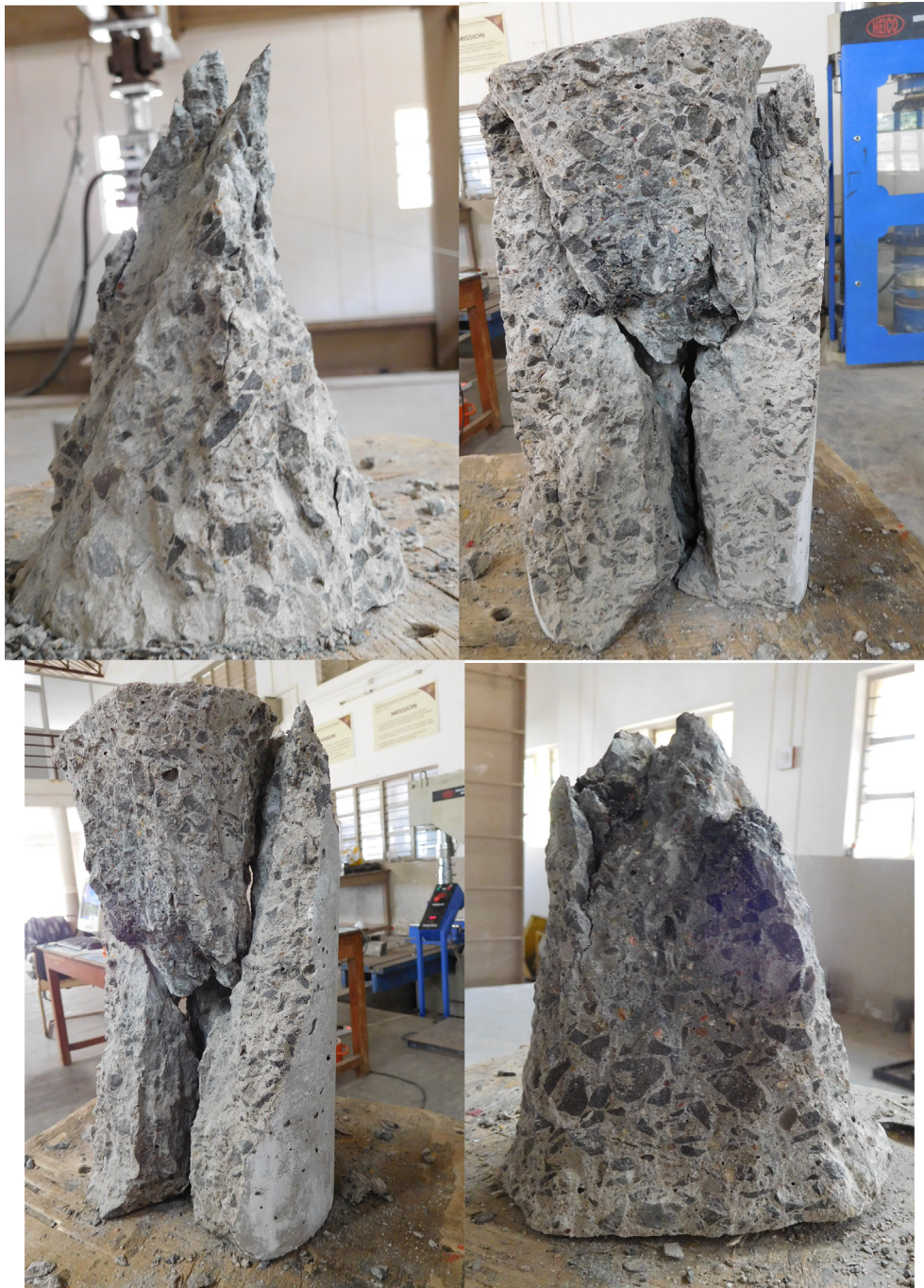
Fig. 11. Failed specimens under cyclic tests.
