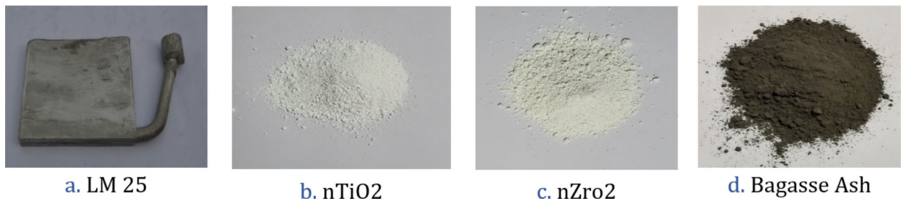
Fig. 1 Filler materials used for casting
