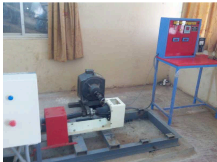
Fig.3 Test rig for fatigue testing of spiral bevel gears.
