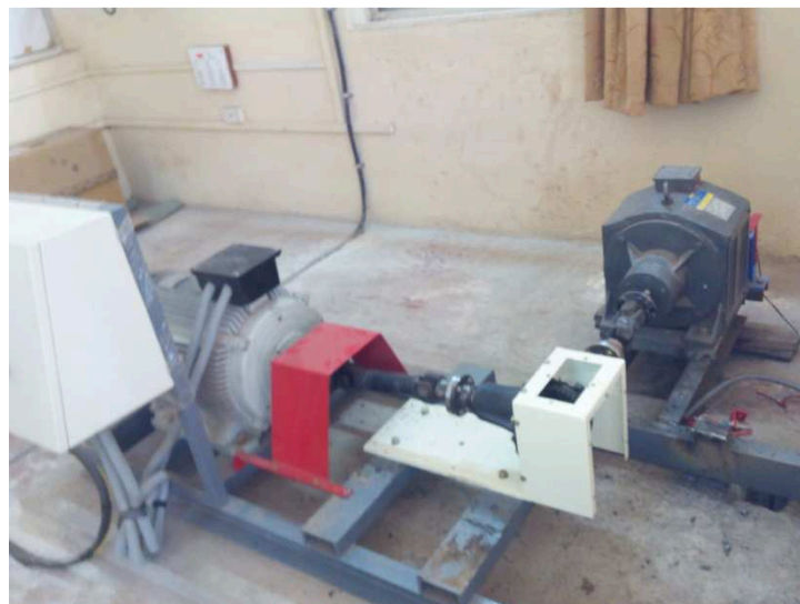
Fig.2 Test rig for fatigue testing of spiral bevel gears.
