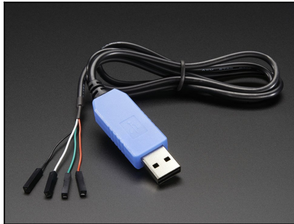
Figure 1.6: A USB to TTL serial console cable. Image courtesy of Adafruit Industries ( https://www.adafruit.com )
