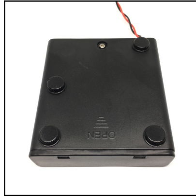
Figure 2.14: Applying the rubber bumpers. Image courtesy of Adafruit Industries ( https://www.adafruit.com ); Image credits—Tyler Cooper
