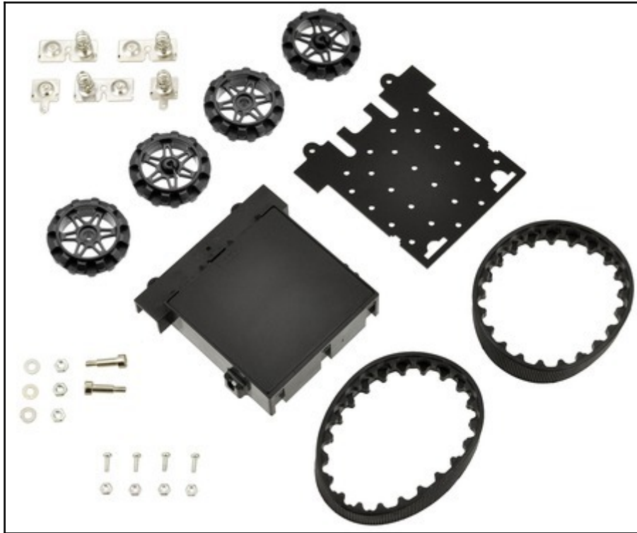
Figure 5.1: Components of the Zumo chassis kit. Image courtesy of Pololu ( https://www.pololu.com/ )
