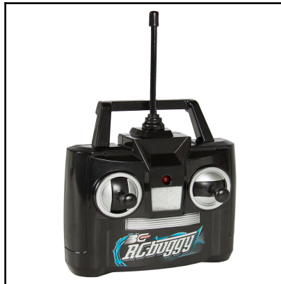
Figure 6.1: A commercial RC Car Remote Controller that can be used to control a hobby car in four directions
