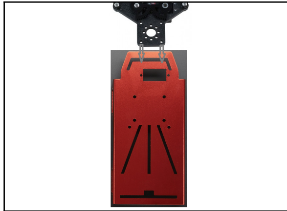
Figure 7.10: Connecting the gripper to the chassis
