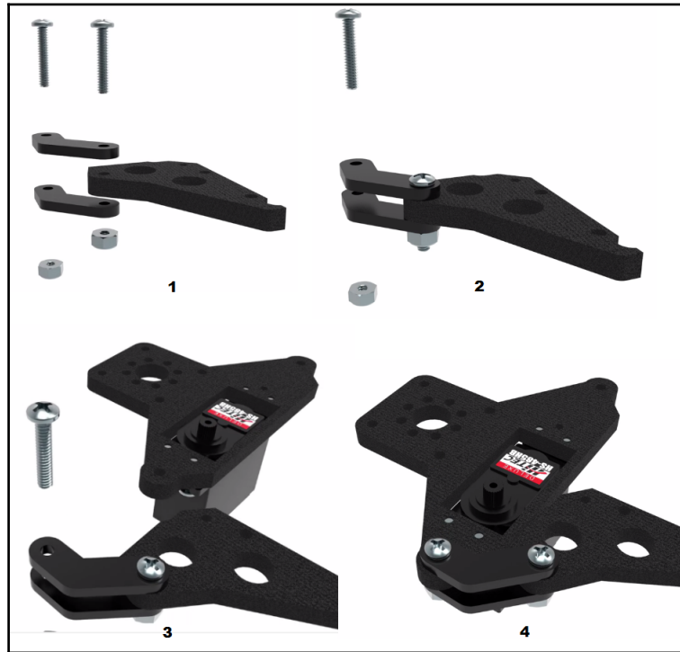
Figure 7.5: Assembling the right-side gripper. Image courtesy of ServoCity ( https://www.servocity.com/parallel-gripper-kit-a )
