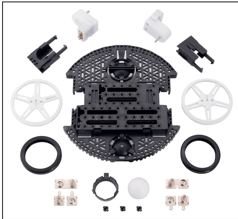
Figure 6.3: Contents of the Romi chassis kit. Image courtesy of Pololu— https://www.pololu.com
