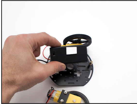
Figure 2.10: Applying a piece of double tape. Image courtesy of Adafruit Industries ( https://www.adafruit.com ); Image credits—John Park
