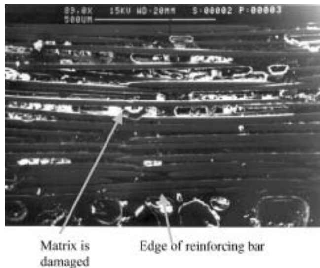
Fig. 6—Damaged area on outer layer of GFRP reinforcing bar (B3-900).
